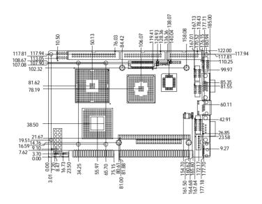
Figure 1.1: Board layout: dimensions (component side)
